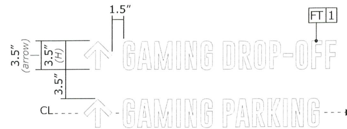
Graphics Layout Schematic | Scale: 1"=1'
