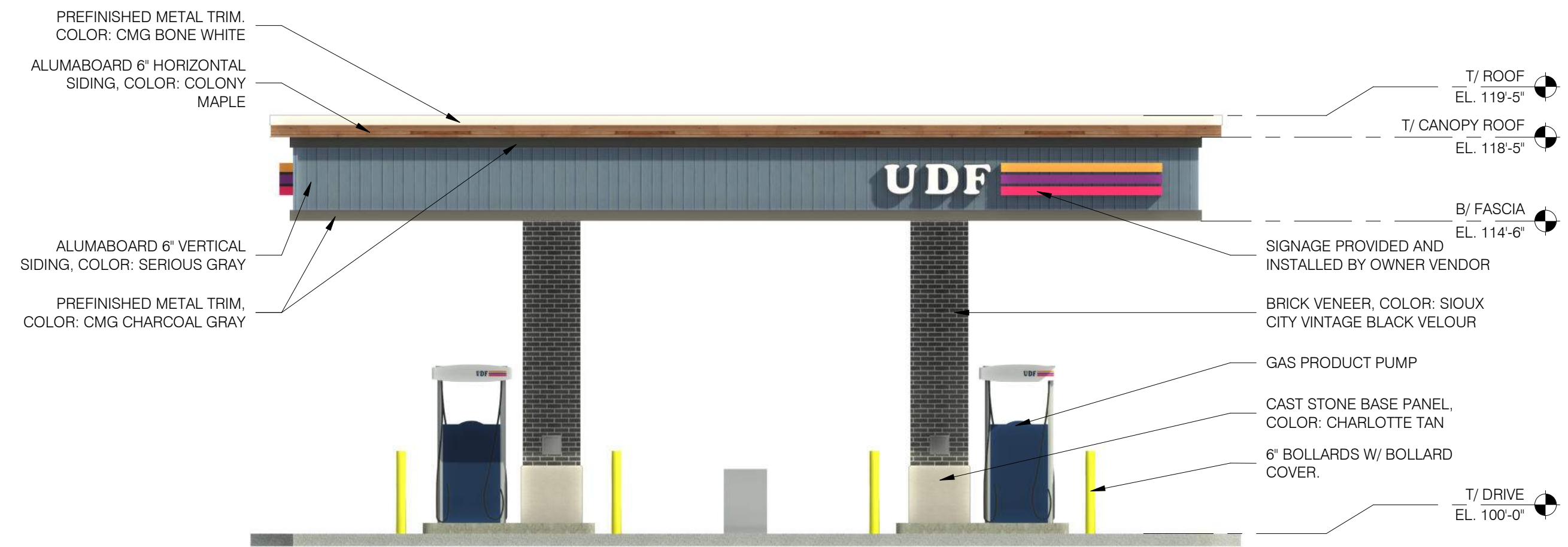
3 GAS CANOPY SIDE ELEVATION SCALE: 3/16" = 1'-0"
